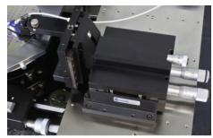
Figure 3. RPP305 positioner on EPS200RF with a solid and stiff probe arm provides accurate probe placement, consistent contact force and overtravel
