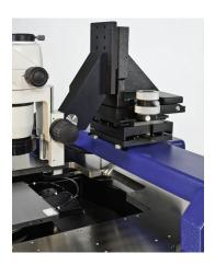
Figure 29. Solid design of the microscope RF bridge and transport with tilt lift
