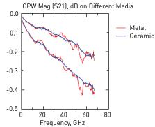
Figure 8. Optimized boundary conditions provided by ceramic AUX chuck improve characteristics of calibration standards
