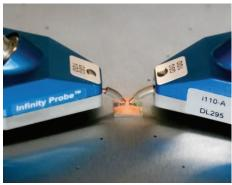
Figure 31. Probing of a single chip on RF chuck
