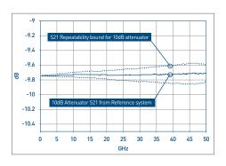
Figure 14. Measurement accuracy verification for a sample DUT calculated by WinCal XE tool
