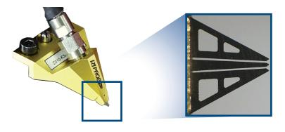
Figure 26. Long MEMS-fabricated coplanar contacts of |Z| Probe provide 200 µm tip compliance and are less sensitive to critical actions
