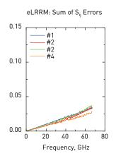
Figure 24. Highly repeatable LRRM calibration available from WinCal XE (included in package)
