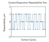
Figure 2. Measured repeatability of the contact/ separation drive over 100 cycles, using EPS200RF with RPP305 positioners
