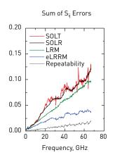
Figure 16. Comparison of different probe-tip calibration methods
