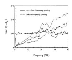
Figure 13. Verification results of probe tip LRRM calibration
